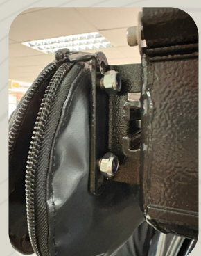
Step 3: Inserting of bolts in mounting holes
